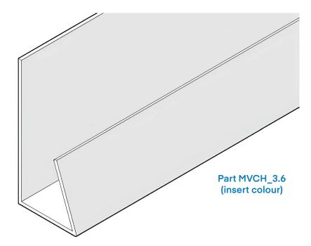
The one-part channel can be used as a universal starting option, around the apron of top storeys that contain raked/sloped rooflines and/or different starting heights or as a vertical trim abutting another cladding. When installed horizontally, 5mm drain holes must be drilled at maximum 600mm centres.
