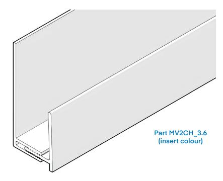
The two-part channel trim can be used as a universal finishing option for both gable ends and horizontal finishes where the weatherboard does not finish on a scallop, around the apron of top storeys that contain raked/sloped rooflines and/or different starting heights or as a vertical trim abutting another cladding providing that the spine of the flashing is not visible.
