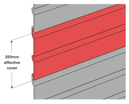
Palliside® is a double-profile weatherboard with a total effective cover of 259mm.
