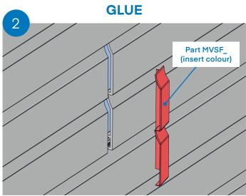
Apply solvent to one side of the back fin of the flat soaker and push in place wiping away excess solvent
