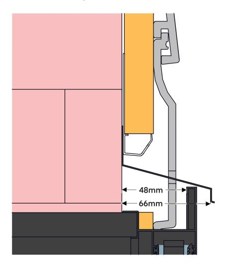
Palliside® finishes require strict adherence to joinery set-out to take into consideration the effect of things like the build-up of flashing tape at corners of openings.
