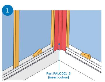
> Ensure the internal corner flashing is straight and true the full length of the corner
