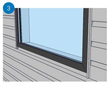
Window shown completed with scriber caps and end plugs installed both sides of joinery.
