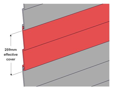
Palliside<sup>®</sup> is a double-profile weatherboard with a total effective cover of 259mm.
