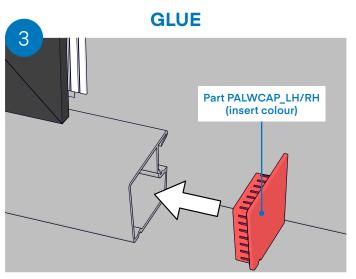
Modify handed sill caps if required (by removing extension tabs) to fit against weatherboard
