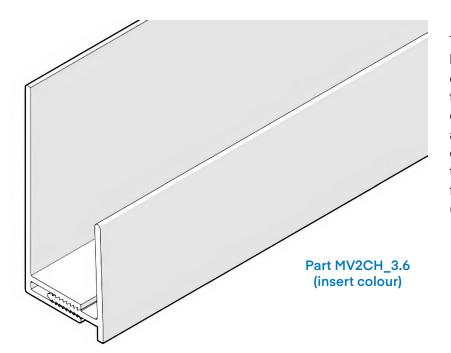
The two-part channel trim can be used as a universal finishing option for both gable ends around the apron of top storeys that contain raked/sloped rooflines or as a vertical trim abutting another cladding. The two-part channel trim cannot be used on horizontal finishes except where modified (refer cut board start).
