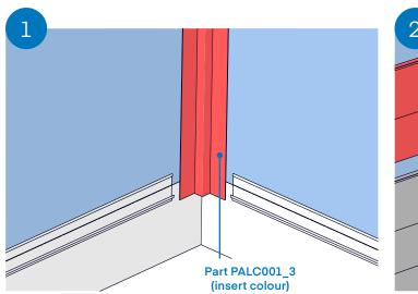
> Ensure the internal corner flashing is straight and true the full length of the corner
