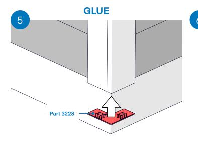
Install bottom box corner cap using solvent cement. Allow a small gap in glue on box cap for drainage.
