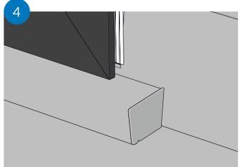
Glue caps each side to sill ends using solvent cement
