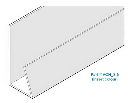
The one-part channel can be used as a vertical trim abutting another cladding but is not ideally suited as a starting option for horizontal part board starts and raked/ sloped rooflines. When installed horizontally, 5mm drain holes must be drilled at maximum 600mm centres.
