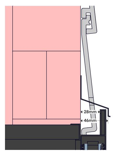
Palliside® finishes require strict adherence to joinery set-out to take into consideration the effect of things like the build-up of flashing tape at corners of openings.
