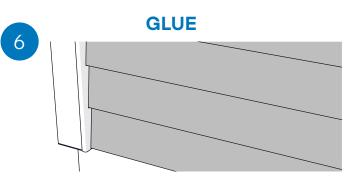
Box corner shown completed with scribers installed both sides and bottom cap to under side.
