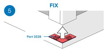
Install bottom box corner cap using solvent cement. Allow a small gap in glue on box cap for drainage.
