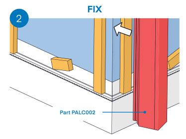
> Check box corner is square & fix through nailing flange
