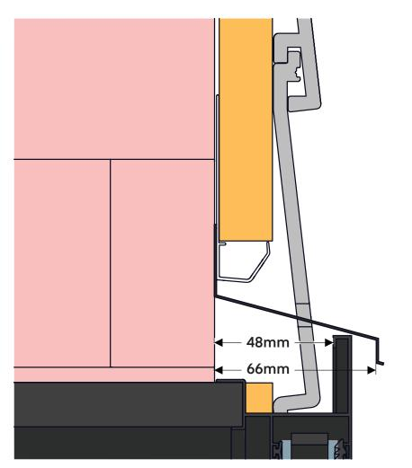
Palliside<sup>®</sup> finishes require strict adherence to joinery set-out to take into consideration the effect of things like the build-up of flashing tape at corners of openings.
