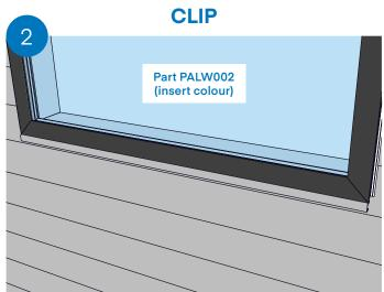
Clip the colour matched cap firmly in place over window base ensuring clip is fully engaged.
