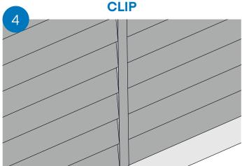
Jointer shown completed with end plugs installed both sides of jointer.
