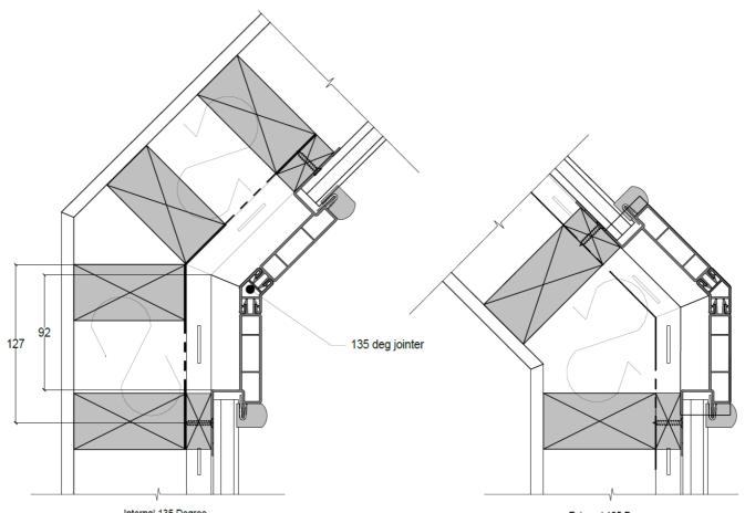
Internal 135 Degree External 135 Degree 135 Degree corners (both internal and external) can be created using the 135 Degree Jointer and 2 male Box Corner components.
